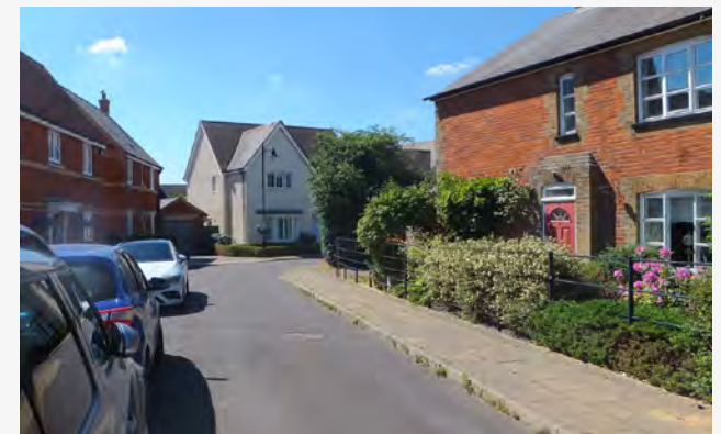
Figure 96: A good level of enclosure can be achieved by a slightly meandering road, small building setbacks and physical boundary treatments, Nonacourt Way.
