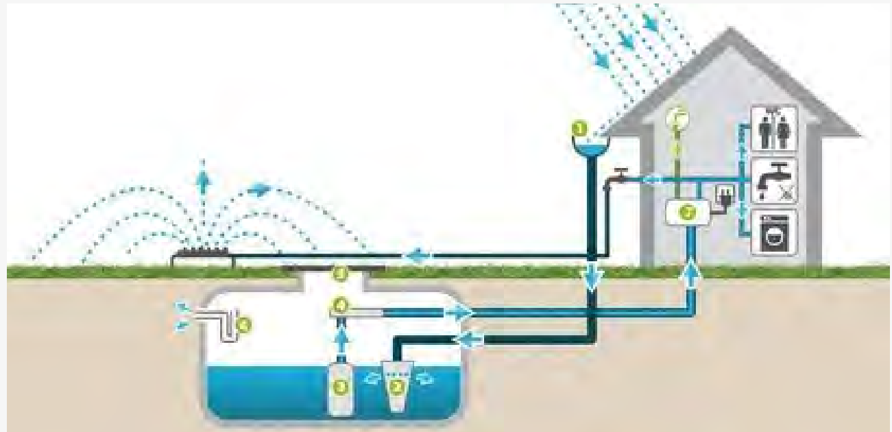
Figure 77: Diagram illustrating rainwater harvesting systems that could be integrated into open space and residential developments.
