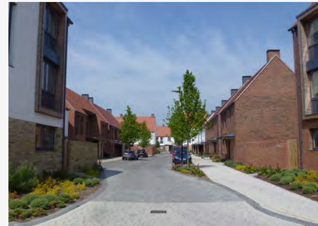
Figure 51: Tertiary street with inset parking bays alternating with trees on both sides in Dewenthorpe, York.
